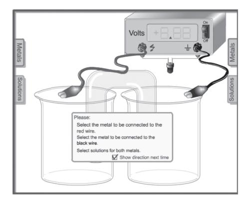
This simulation contains an apparatus for measuring the voltage generated by chemical reactions. This apparatus is called a voltaic cell. Pop-out menus will allow you to select metals (electrodes) and ionic solutions to be placed into two beakers that are connected by a salt bridge. You can then connect the metals to a voltmeter to measure the cell voltage ( $E^\circ$ ).
