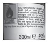
The container is a constant volume environment. Temperature is directly proportional to pressure, so any increase in temperature will also increase the pressure in the container. The warning reflects a maximum temperature above which, testing has established , the particular type of container could fail, suddenly releasing the gas in an explosion.
