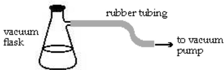
The vacuum flask side arm has vacuum rubber tubing with one end attached to the flask and the other end attached to a vacuum pump (can not see in this diagram). When the vacuum pump is on any gas/vapor in the flask is removed.
